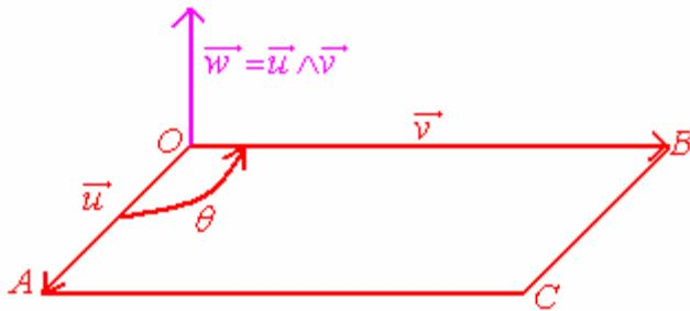
$$\begin{aligned} s &= \frac{1}{2} OA \times OB \times \sin(\theta) \\ s &= \frac{1}{2} \|u\| \times \|v\| \times \sin(\theta) \\ s &= \frac{1}{2} \|u \wedge v\| \end{aligned}$$
